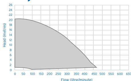
The shaded performance range curve above illustrates the ability of the pump to deliver varying flow rates at a variety of different speed settings. The main factor that determines how much flow is delivered from your pump is the amount of restriction (friction) in the line. This is represented in head and measured in metres.
